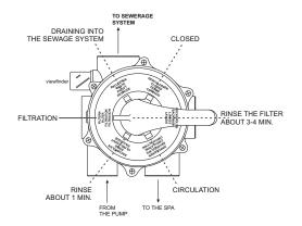
FILTERN, FILTER, FILTRATION, FILTRACION - filtration (normal operation)
