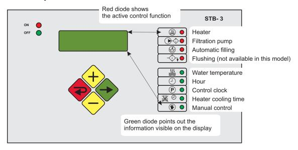
STB-3 system will once a week control the temperature, the water level and the filtrating process of the SPA bath.
