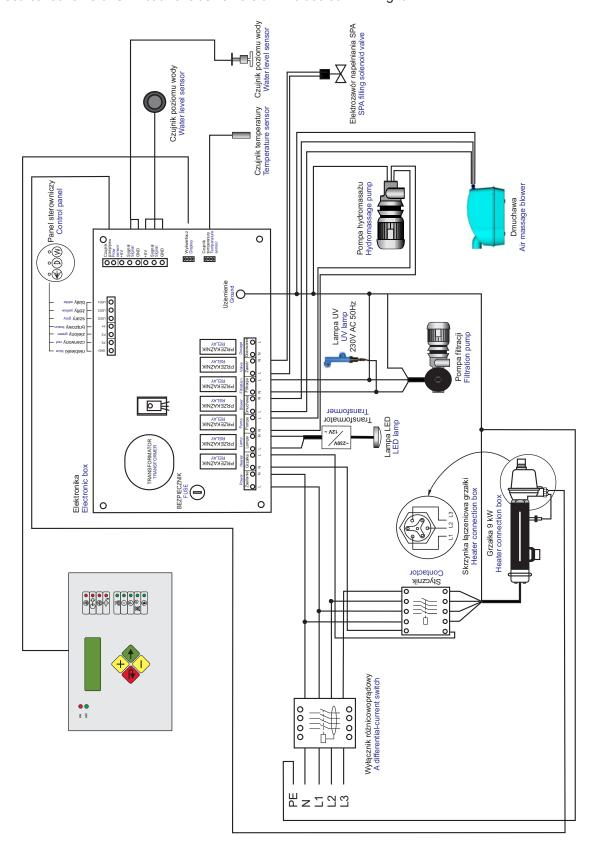
Fig. 3a. Electrical scheme of SPA bath exclusive version: LED spotlight – 24 points
