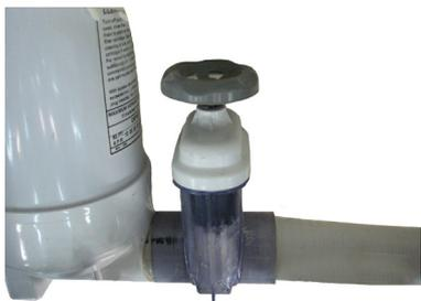
In the Genesis SPA bathtub there are **5** slide valves that disconnect the water flow to the pump and the heater. Closed valves make it possible to inspect, repair or replace devices with a filled bathtub.
