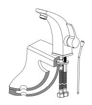
Insert the lift pole 9 through the hole at the back of the faucet body 1.
