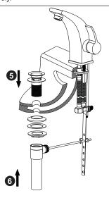
Insert the drain-off pole 10 through the hole of the basin. Tighten the drain-off pole 10 securely. Place the end side of the lift pole 9 through the drain-off pole 10 and then tighten the screw.
