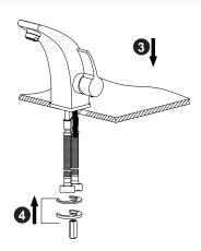
Insert waterlines 3 and fixing bolt 2 into the set hole of the under mount sink or 1 3/8"drilled hole of the counter top. Put on the rubber washer 5 and brass washer 6 then securely tighten with nut 7. Place the faucet body 1 and use the spanner to tighten the nut 7 securely.
