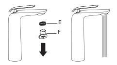
Remove adjustable aerator (E) with aerator key (F). Turn water on for 1 minute to remove any debris. Reassemble adjustable aerator (E)
