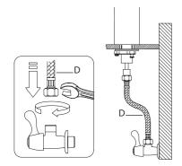
Thread hot & cold waterlines (D) onto angle stops and tighten with adjustable wrench until snug. Turn on angle stops and check for leaks (DO NOT TURN ON FAUCET)
