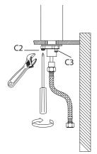
After adjusting direction of faucet body (A), tighten mounting nut (C2) with adjustable wrench. Secure mounting nut (C2) by tightening mounting screws (C3) with a Phillips head screwdriver
