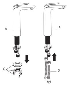
Remove mounting hardware (C) from faucet body (A). Place faucet body (A) on a soft cloth. Secure hot & cold waterlines (D) at the base of the faucet (handtighten, then secure with ¼ turn of adjustable wrench) A. Hot Side: Left B. Cold Side: Right
