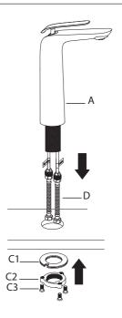
Install faucet body (A) through 1 3/8" hole in countertop, with base O-ring (B) and hot & cold waterlines (D) attached. Attach rubber & metal O-washer (C1) and mounting nut (C2) to threaded mounting pipe
