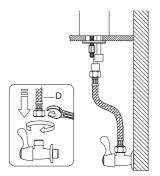
Thread hot & cold waterlines (D) onto angle stops and tighten with adjustable wrench until snug. Turn on angle stops and check for leaks (DO NOT TURN FAUCET ON)
