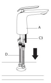
Remove faucet, mounting hardware, and waterlines from the box. Remove mounting nut (C4) from mounting screw (C3). Place faucet body (A) on a soft cloth, spout facing up. Secure hot & cold waterlines (D) at the base of the faucet (hand-tighten, then secure with 1/4 turn of adjustable wrench) A. Hot Side: Left B. Cold Side: Right Thread mounting screw (C3) into faucet base, flat head up, and tighten with a Phillips head screwdriver until snug
