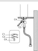
Install rubber U-washer (C1) and metal U-washer (C2) from underneath the countertop or sink. Attach mounting nut (C4) to mounting screw (C3) and tighten with adjustable wrench or 10mm wrench until snug
