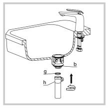
• Thread tailpipe (h) onto drain (b) and hand-tighten. Adjust tailpipe (h) so drain off pole opening is to the rear of the sink
