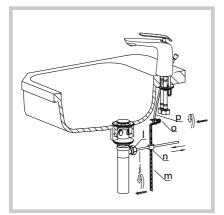
• Place one end of clip (n) on drain off pole (j). Insert drain off pole (j) through desired hole of extender rod (m). Place other end of clip (n) on drain off pole (j)
