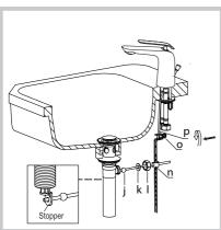
• Insert shortest end of drain off pole (j) into drain off pole opening of tailpipe (h). Make sure drain off pole (j) and slot on waste stopper (a) engage. Attach washer (k) and retaining nut (l) through drain off pole (j). Secure retaining nut (l) to drain off pole opening of tailpipe (h)
